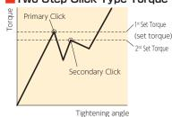
The primary 'click' sound signals reaching the 1st set torque and the secondary click signals tightening completion. Tightening after the 2nd click causes over-torque. Compared with the click type, Two-Step Click Type leaves wider margin after clicking and is more effective against over-torque.
