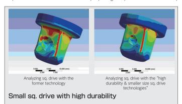
Applying various technologies such as FME (Finite Element Method), Tohnichi has succeeded to develop the smaller size square drive, interchangeable head, and torque wrench (applied to QL25N5-1/4, QL100N4-3/8, QL280N-1/2 and interchangeable heads QH series). This enables our torque wrench to use with the smaller size socket, so that eventually devotes to decrease the total weight of the tool, and leads to increase users' workability.
