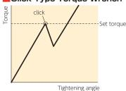
The most standard torque wrench. A clear 'click' sound signals tightening completion upon reaching the set torque. Once recognizing the clicking sound and feeling, stop to apply force and finish tightening to avoid over-torque.
