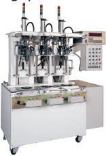
On this machine each spindle will tighten individually one by one, stopping automatically at the preset torque value. At the same time the machine will check the tightening torque value and perform OK-NG judgment automatically. It features provisional tightening control, work piece model selection, and detection of product defects. The measured data can be transferred to a computer for data processing.
