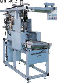
When the work piece is set in front, it is automatically transferred to the back, where bolts on the upper face and side faces are automatically tightened. When the tightening is completed, the lamp will light and the work piece will return to the original position.
