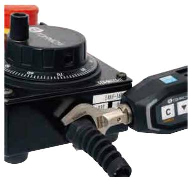
For tightening in narrow areas where height and other restrictions make it difficult to tighten with a torque screwdriver or conventional torque wrenches.
